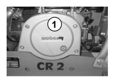
Check the V-belt (1) for cracks, damaged flanks, and wear. If there is excessive wear – replace the V-belt as specified in the repair manual.
