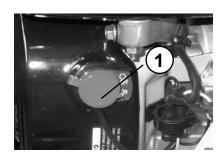
Slide the choke lever (1) to the left (close). Open the fuel cock (2).
