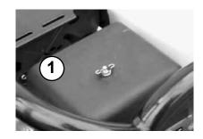
Remove the air filter insert (1) from the air filter enclosure. Clean air filter insert as specified by the engine manufacturer if there is damage or if it is extremely dirty.
