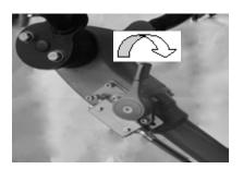
Turn the short-circuit button (1) to the "ON" position.
